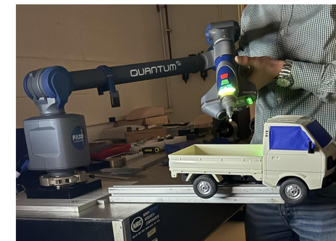
Figure 7. Faro laser scanning
