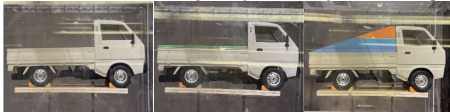
Figure 2. Truck bed configurations in wind tunnel. Open bed (left), flat cover (middle), and sloped cover in (right).
